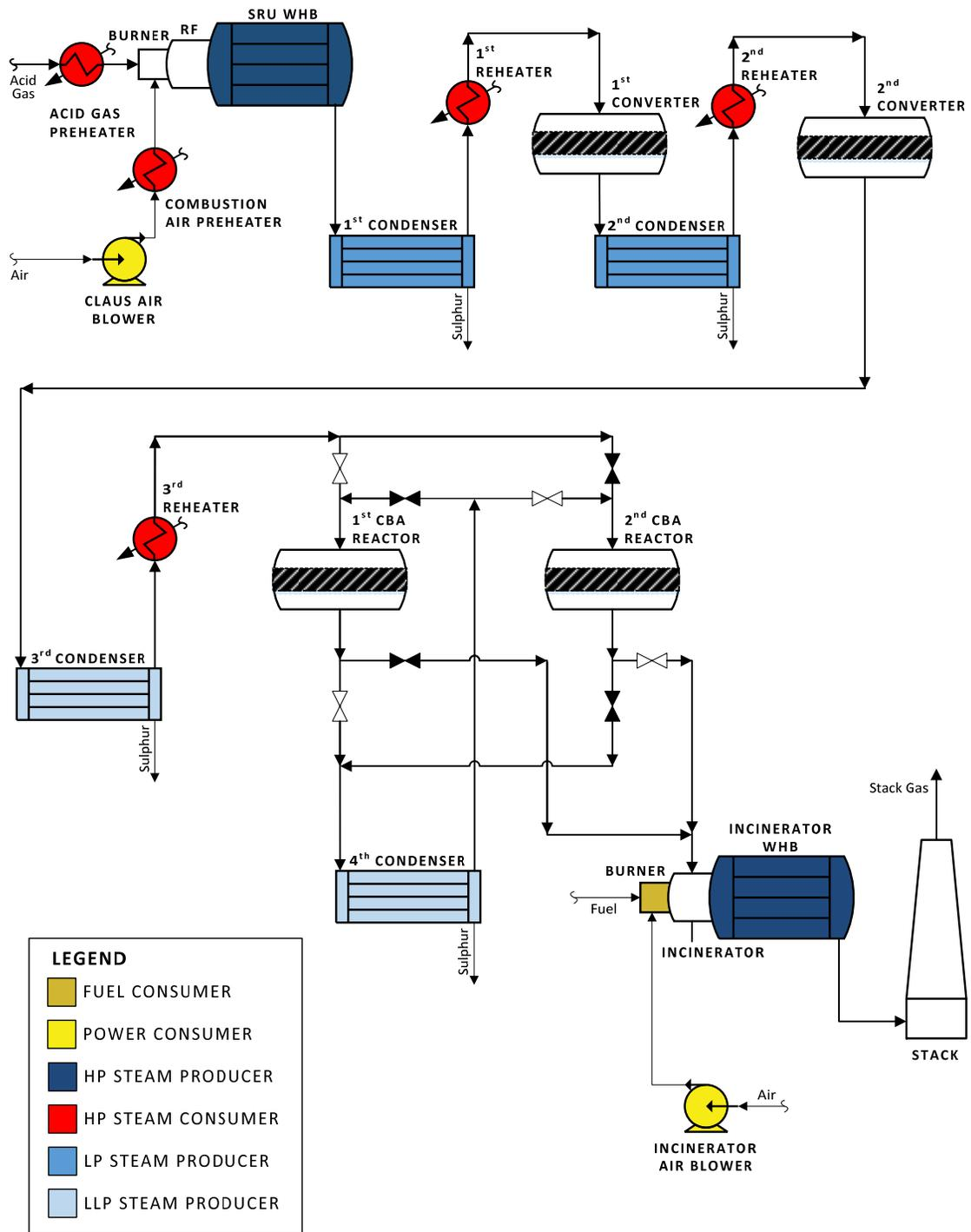
Figure 5. PFD for Benchmark Plant Cases C and D
