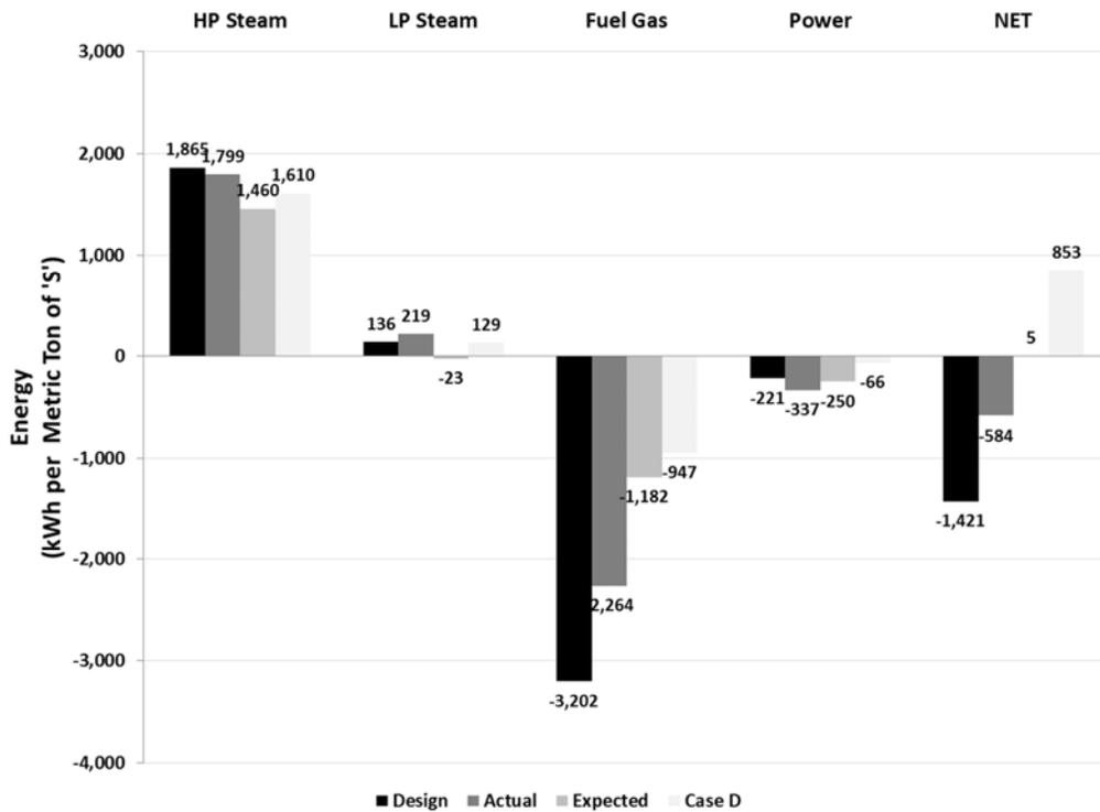
Figure 8 illustrates fuel gas consumption KPIs by major equipment and shows that fuel consumption in the combustion air preheater, co-firing in the SRU burner and RGG contribute significantly to overall fuel gas requirements in the Real World Plant. For the Benchmark Plant Case D, these fuel gas consumers are not required, resulting in a considerably lower fuel consumption KPI. In all cases, the incinerator is a significant fuel consumer.
